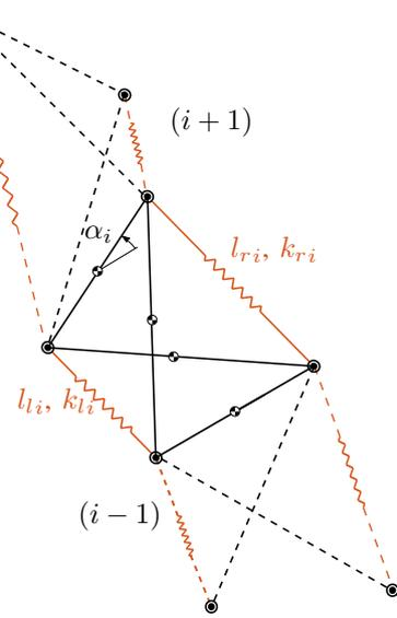
Fig. 1: Parametrization of a stack of mechanisms.
