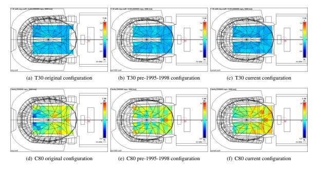
Figure 3. Reverberation time T30 and Clarity C80 simulation results for 1 kHz-octave band. 500000 rays used, ray truncation time 3000 ms.
