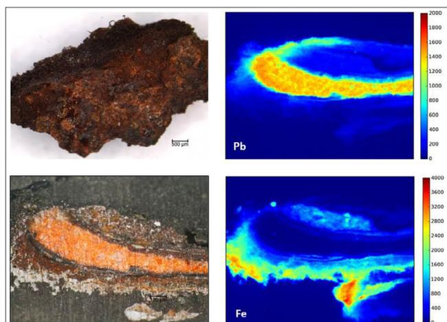
Figure 3. Paint flake sample from the measuring and cross-section series observed under optical microscope and XRF maps of major elements
