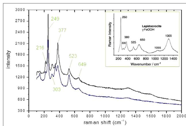
Figure 4. Raman spectra of corrosion products acquired at two points of interest on the sample from the series of measures
