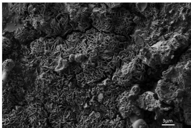
Figure 2. SEM image (SE mode, 2 keV) of the corrosion products formed between the metal and the paint layers of the sample collected from the weighing scale
