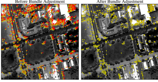
Figure 2: Effect of pointing error before and after bundle adjustment. Green dots represent the detected features, and red vectors the distance to the reprojected locations (i.e. reprojection error). After bundle adjustment, the reprojection error reaches subpixel magnitude, implying that the RPCs have been corrected.
