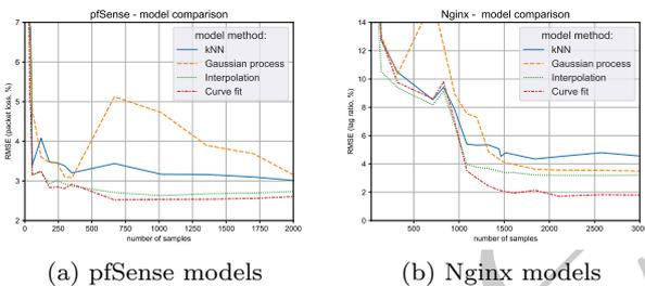
**Fig. 12** Comparison of the prediction accuracy of different methods trained with the same sampled dataset.
