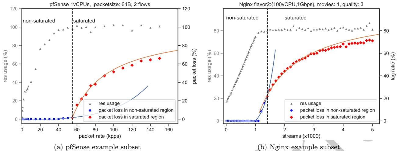
**Fig. 3** The Curve fit model exemplified in two example VNF subsets. For each plot, the y-axis on the left is for the saturating resource usage, the one on the right depicts the increasing KPI value. The boundary between (non) saturated regions is where the workload covariance with the KPI becomes larger than with the resource usage.
