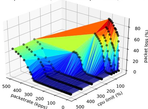
**Fig. 6** A subset of the pfSense dataset to illustrate the response surface of the KPI (packet loss), under different vCPU allocations.
