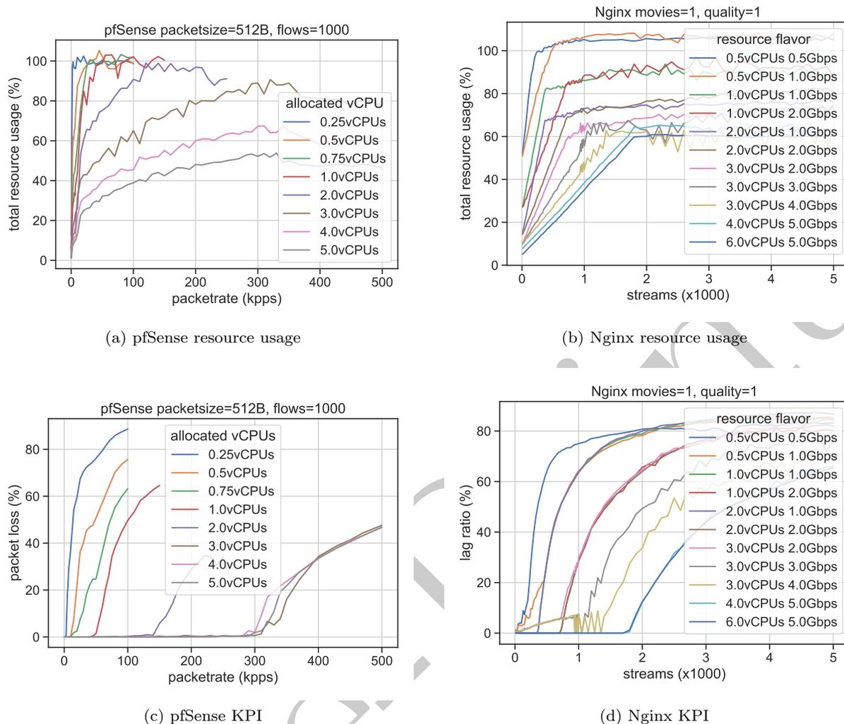
**Fig. 2** Subset of measured VNF metrics under different resource allocations.
