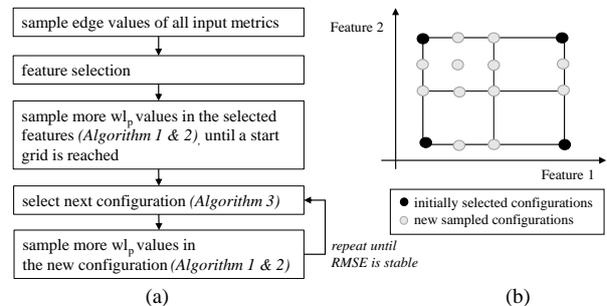
**Fig. 10** (a) The sampling workflow with (b) simplified representation of the sampled configuration space.
