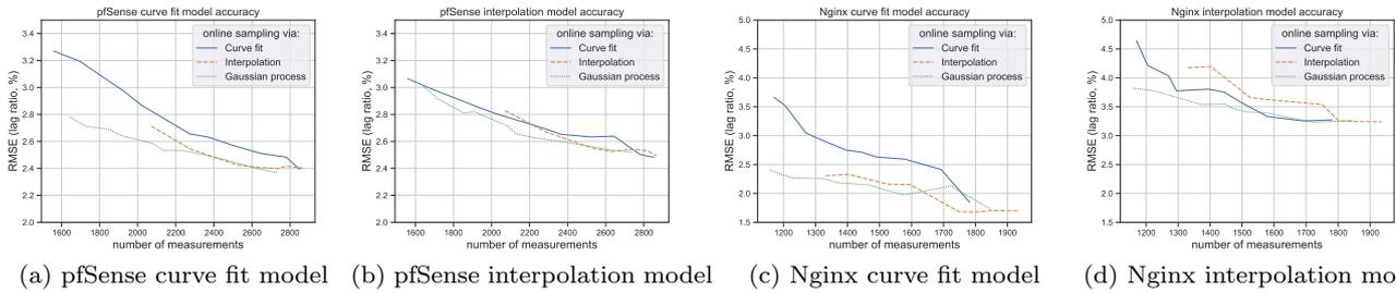
**Fig. 8** When sampling the workload metric  $wl_p$  online, a Gaussian Process (GP) works best to assess when enough samples are taken. The GP produces the best model for the KPI trend, under varying  $wl_p$  values, and with the least amount of samples.
