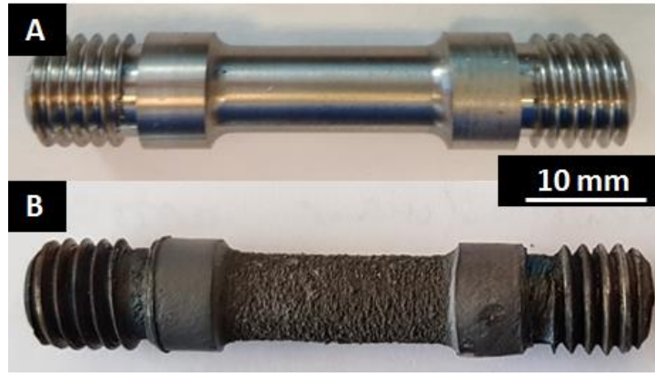
Fig. 1 Experimental sample before deformation (A) and after deformation at 1050°C and 0.5/s (B)
