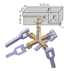
Fig. 5: Milling as a tentative application of the 4-rRUU PM prototype.
