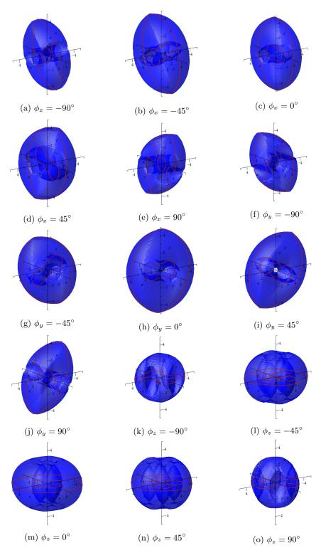
Fig. 2: Workspaces of  $4\text{-}R_xUU(\text{a-e}),\,4\text{-}R_yUU(\text{f-j})$  and  $4\text{-}R_zUU(\text{k-o})$  PMs
