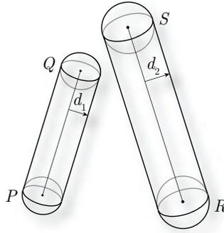
Fig. 3: Link interferences as collision between two capsules
