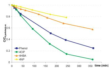
**Figure 2.** Normalized concentration-time profiles of the phenols during batch CWAO on F22, after stabilization of AC activity ( $p_{0_2} = 3.5$  bar, T = 150 °C, initial concentration of 1 g·L<sup>-1</sup> for each pollutant) ( $C_{0,ox}$  refers to the concentration after adsorption).
