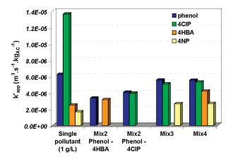
**Figure 4.** Apparent oxidation rate constants ( $k'_{app}$ ) calculated after stabilization of AC activity according to  $R_{pol,app} = k'_{app}C_{pol}$  for the different compound mixtures studied ( $p_{O_2} = 3.5$  bar, T = 150 °C, initial concentration of 1 g·L<sup>-1</sup> for each pollutant, F22 carbon).
