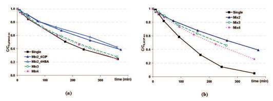
**Figure 3.** Normalized concentration-time profiles of the considered pollutant (single or in mixtures) during batch CWAO over F22, after stabilization of AC activity ( $p_{02} = 3.5$  bar, T = 150 °C, initial concentration of 1 g·L<sup>-1</sup> for each pollutant): (a) phenol, (b) 4-chlorophenol (4ClP) ( $C_{0,ox}$  refers to the concentration after adsorption).
