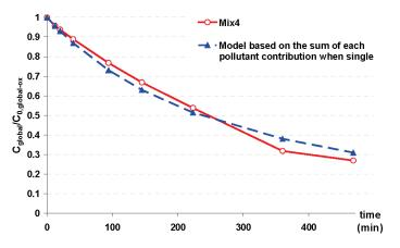
**Figure 5.** Time-evolution of the normalized global molar concentration of Mix4 during batch CWAO over F22, after stabilization of AC activity ( $p_{O_2} = 3.5$  bar, T = 150 °C, 1 g·L<sup>-1</sup>, initial concentration of 1 g·L<sup>-1</sup> for each pollutant).  $C_{0,ox}$  refers to the concentration after adsorption. Model:  $C_{global} = \sum_{\substack{c mix4 \\ comta = 0}} C_{0,i-ox} \cdot \exp(-(k'_{app,i})_{single}(w_{AC}/V_L)t)$ .
