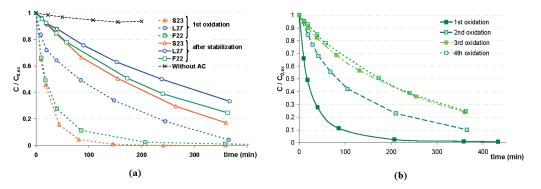
**Figure 1.** Normalized phenol concentration-time profiles during CWAO of phenol ( $p_{02} = 3.5$  bar, T = 150 °C,  $C_{ini} = 1$  g·L<sup>-1</sup>): (a) initial and stabilized performance of the investigated carbons, (b) successive oxidations with recycling F22. ( $C_{0,ox} = C_e$  refers to the concentration after adsorption).
