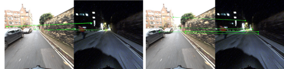
(a) Standard sparse-to-sparse matching using SuperPoint detections and two different descriptors : (Left) SuperPoint descriptors [4 inliers], (Right) HyperColumn descriptors [5 inliers]
