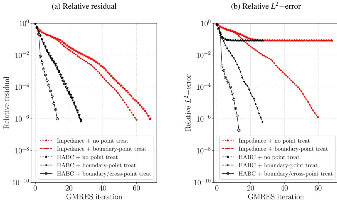
Figure 3: Scattering benchmark: History of residual (a) and  $L^2$ -error between the DDM solution and the monodomain numerical solution (b). The transmission operators are based on the basic impedance condition (red lines) or the HABC (black lines), with and without boundary/cross-point treatments. Parameters:  $N = 4$  and  $\phi = \pi/3$
