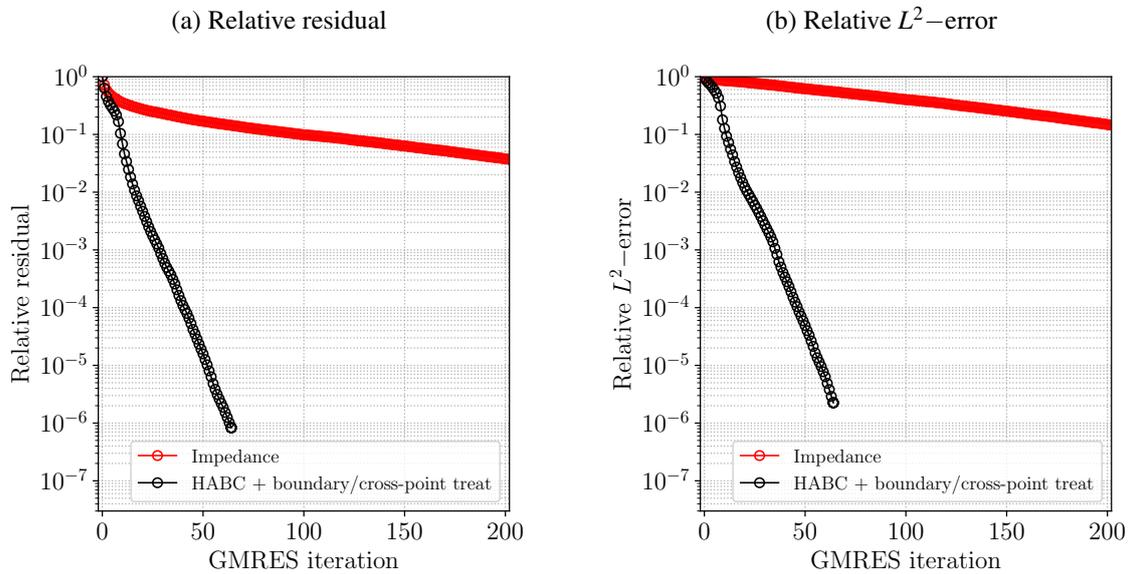
Figure 5: Marmousi benchmark: History of residual (a) and  $L^2$ -error (b) for transmission operators based on the basic impedance condition (red lines) or the HABC (black lines) with point treatments. Parameters:  $N = 4$  and  $\phi = \pi/3$
