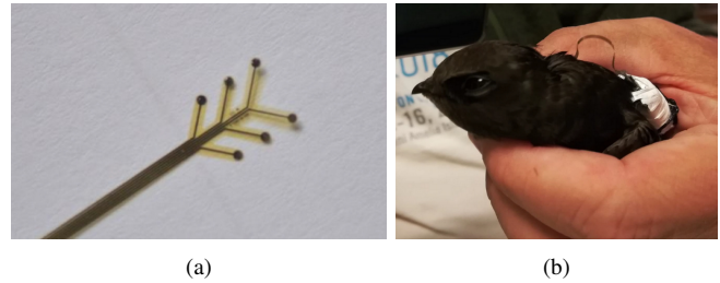
Fig. 6. (a) Flexible printed electrodes array for subcutaneous EEG and (b) picture of a common swift with the system attached to its back.
