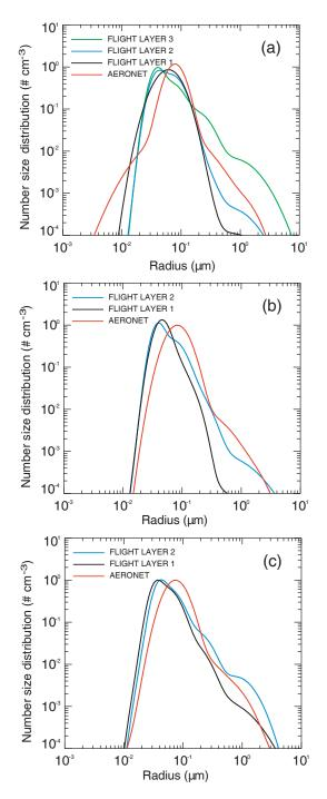
**Figure 4.** Normalized aerosol number size distribution derived from AERONET measurements (red curve) and from the airborne in situ measurements for the layers of Fig. 3 for (a) F35, (b) F38, and (c) F42.
