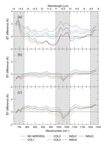
**Figure 12.** Differences between modelled and measured IASI BT spectra at the TOA for (a) 22 June, (b) 28 June, and (c) 3 July. Simulations have been performed with different AOPs and sampled at  $15 \text{ cm}^{-1}$  intervals. The vertical black dashed lines delimit the two spectral intervals (780–980 and 1070–1200 cm<sup>-1</sup>) where the differences are discussed, while the shaded areas are not considered in the analysis.
