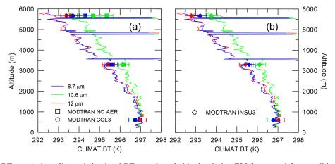
Figure 7. CLIMAT BTs vertical profiles and simulated BTs at selected altitudes during F35 for aerosol-free conditions and with different AOPs: Algerian and Moroccan dust RIs with (a) AERONET, and (b) in situ PSD.
