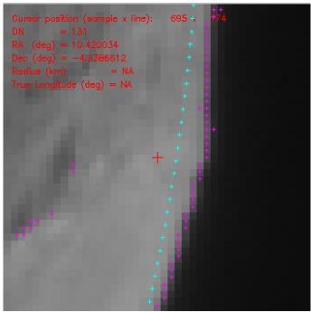
**Fig. 6.** Zoom of the area enclosed by the white box at the upper right in Fig. 4, showing how the measured limb (magenta) departs from the ellipsoidal model (cyan) due to the distorting effect of the crater rim.
