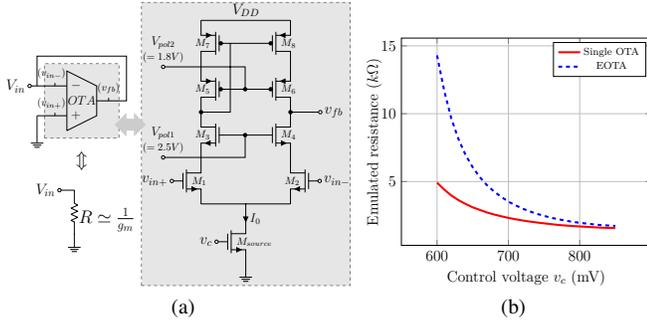
Fig. 2. (a) Resistor implementation using an OTA [16] on the left and its CMOS telescopic cascode implementation on the right (b) Emulated resistance as a function of  $v_c$  using a single OTA (red plain line) and a EOTA (blue dotted line) configured as in (a)
