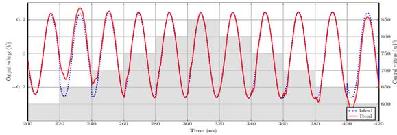
Fig. 5. Simulation of the phase-shifter output  $V_{out}$  for transient variations of the control voltage  $v_c$  (represented as shaded background)
