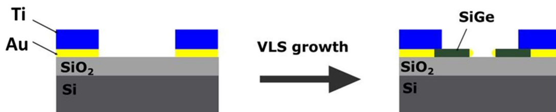
Figure 1: Schematic illustration of a direct growth SiGe NW between two predefined deposited and patterned electrodes.
