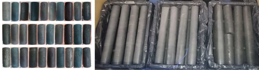
Fig. 1. Left: Condition of specimens after each freeze-thaw exposure cycle (high: water, centre: gypsum water, down: acid water) - Right: Illustration of the conservation of the cores immersed in the trays placed in the thermo-regulated boxes during a test in isothermal condition (left: water, centre: gypsum water, right: acid water).
