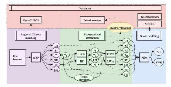
**Figure 2.** Simulation workflow. Squared boxes represent modeling steps and rounded boxes represent meteorological variables. Variables that are not inputs or outputs of a model are indicated by dotted lines (see a glossary of abbreviations used in Appendix A).
