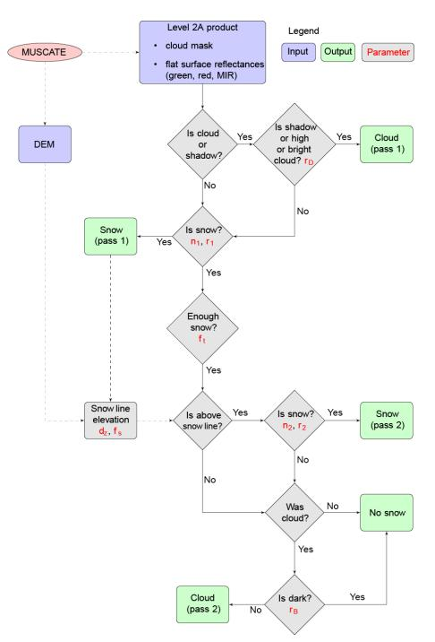
**Figure 3.** Flow chart of the snow detection algorithm. Table 1 gives the description and value of the algorithm parameters (written in red in this chart). MUSCATE is the scheduler which manages the L2A production for Theia.
