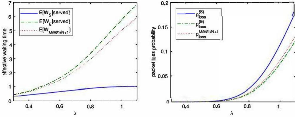
Fig. 6. Mean waiting time (left) and loss probability (right) of the STPQ with  $N = 10$ ,  $\mu = 1$  and  $\alpha = 0.3$ . The arrival rate is  $\lambda = \lambda_S + \lambda_E$  with  $\lambda_S/\lambda_E = 0.2$ .
