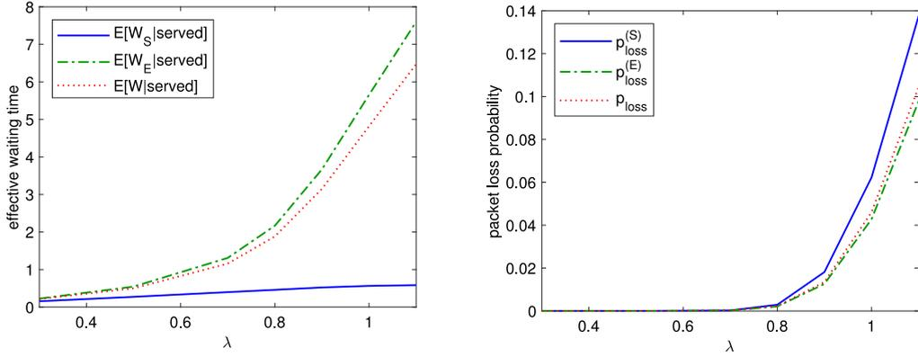
**Fig. 11.** Mean waiting time (*left*) and loss probability (*right*) of the STPQ with  $N = 10$ , deterministic service times (size 1) and  $\alpha = 0.3$ . The arrival rate is  $\lambda = \lambda_S + \lambda_E$  with  $\lambda_S/\lambda_E = 0.2$ .
