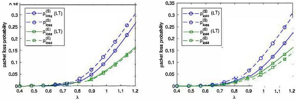
Fig. 8. Light-traffic approximation performance over loss probabilities for both class-S and class-E packets on a system with parameters  $N = 10$ ,  $\mu = 1$  and  $\alpha = 0.8$ . The arrival rate is  $\lambda = \lambda_S + \lambda_E$  with proportions satisfying (left)  $\lambda_S/\lambda_E = 0.15$  and (right)  $\lambda_S/\lambda_E = 0.3$ .
