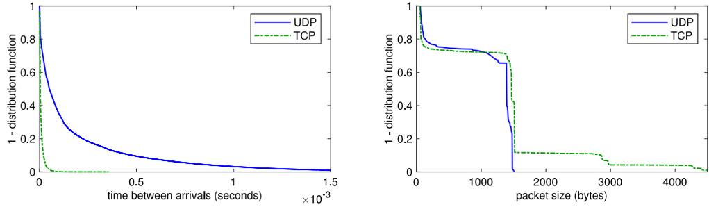
**Fig. 12.** Complementaries of the cumulative distribution functions of seconds between packet arrivals (*left*) and size of packets in seconds (*right*) of the real trace of 5 million packets considered to simulate the STPQ.
