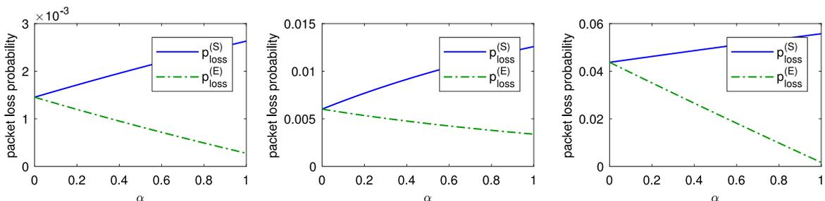
**Fig. 5.** Loss probabilities for the STPQ with parameters  $N = 10$  and  $\mu = 1$  with respect to the push-out probability  $\alpha$  for different traffic configurations.  $\lambda_S = \lambda_E = 0.3$  (left),  $\lambda_S = 0.2, \lambda_E = 0.5$  (center) and  $\lambda_S = 0.7, \lambda_E = 0.2$  (right).
