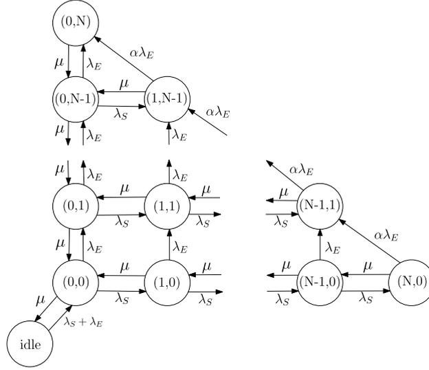
Fig. 1. State transition rate diagram for the STPQ.
