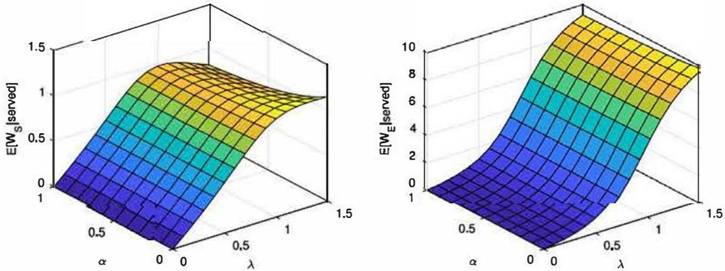
Fig. 7. Mean waiting time for class-S (left) and class-E (right) packets with  $N = 10$ ,  $\mu = 1$  and a proportion of traffic  $\lambda_S/\lambda_E = 0.25$ , with total arrival rate  $\lambda = \lambda_S + \lambda_E$ .
