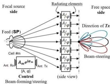
Figure 1: Principle of a transmit-array in transmit mode
