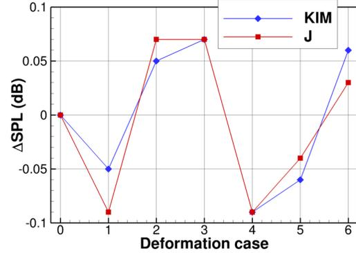
Figure 3: Loading noise SPL variations obtained by  $KIM$  and the acoustic function  $J$ , at the BPF and in the propeller plane, with local blade deformations: 0: no deformation; 1-2: sweep  $\pm 2^\circ$ ; 3-4: chord  $\pm 2\%$ ; 5-6: thickness  $\pm 2\%$
