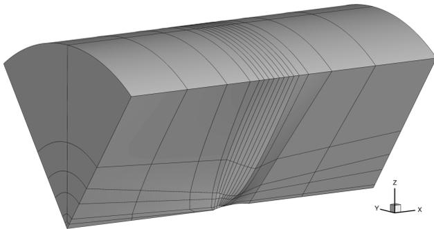
Figure 1: Mesh blocks of the CFD domain
