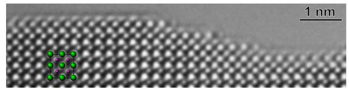
**Figure 2.** Experimental HR(E)TEM [001]-CeO<sub>2</sub> image in 'white atom' contrast acquired under environmental conditions ( $P(CO_2) = 7 \cdot 10^{-1}$  mbar). The image shown was obtained after realignment of a stack of 100 4kx4k frames recorded at 10 fps and averaged to improve the SNR. Inset: Ce(large green dots); O(small purple dots).
