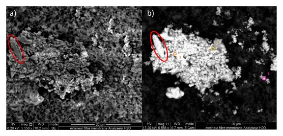
**Figure 5.** Observation of a large particle (>7  $\mu$ m) formed by the agglomeration of smaller particles of different sizes and shapes at ×5556 magnitude with detectors secondary electrons SE (**a**) and backscattered electrons BSE (**b**).
