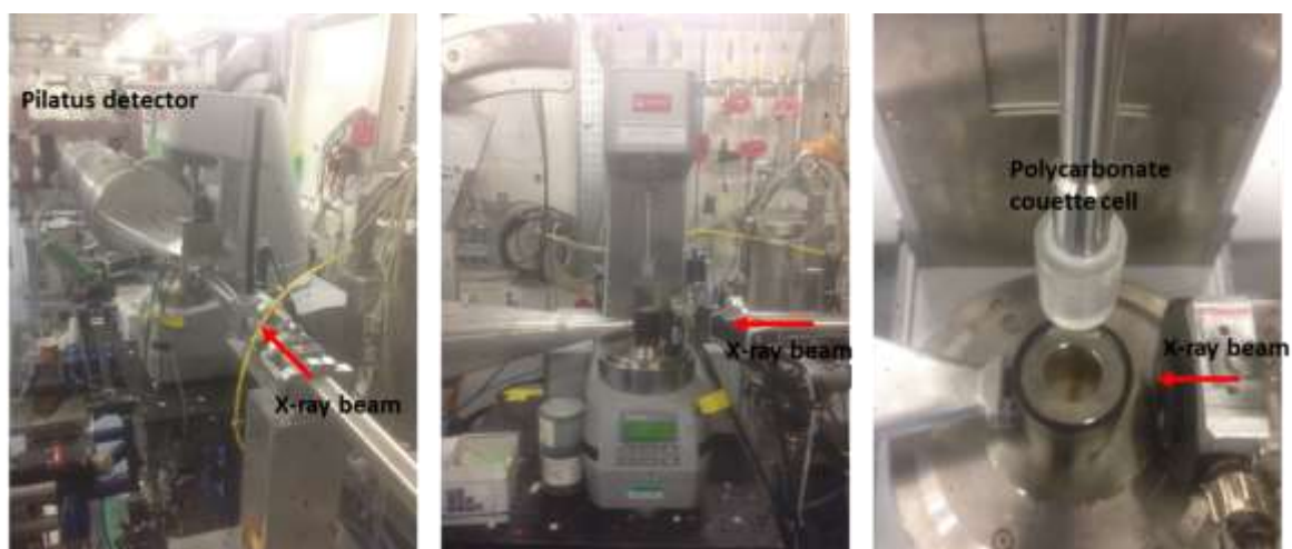
Figure S 6 – Rheo-SAXS apparatus used at the BM29B beamline at ESRF synchrotron (Grenoble, France). A MCR 501 rheometer (Anton Paar, Graz, Austria) equipped with a Couette polycarbonate cell (imposed gap = 1 mm) is employed. A radial configuration is used during the Rheo-SAXS study.
