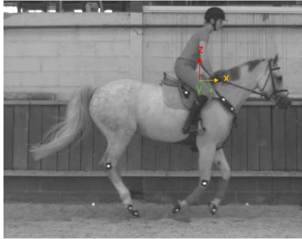
Figure 1: Orientation of IMUs axes on an equipped horse
