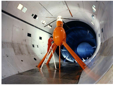
Fig. 1: 7A rotor mounted in ONERA Modane SIMA Wind Tunnel.
