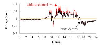
Fig. 10. Daily voltage profile of the PV generator in node #18 (CASE#1).
