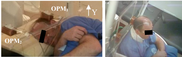
Fig. 7: Experimental setup used during Auditory Evoked Fields (AEFs) (left part), Visual Evoked Fields (VEFs) and alpha rhythm recordings (right part) carried out with OPMs
