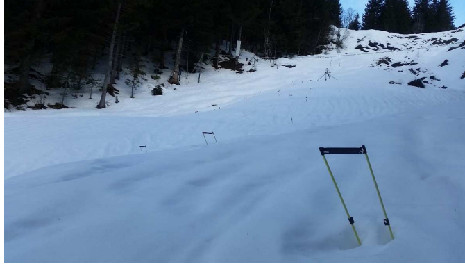
Fig. 11. Photo illustrating the two main sources of inaccuracies in this experiment the snow (particularly the first snowfall) and the angle of the tag supports, which created a reversible error of 4.9 cm ( 3\sigma ) at the end of October and a slow drift roughly estimated at up to 5 cm per month, respectively. Apart from those two specific problems, the accuracy remained below 1.1 cm ( 3\sigma ).
