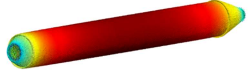
Figure 11: Surface magnetic flux density of a submarine model with 33.298 surfaces elements, 83.245 branches, and 49.947 independent loops, solved in 12 min (i5-6600, 6GB DDR3) with a matrix compression ratio of 89.5 % (ACA).
