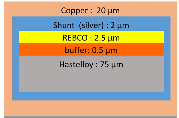
Fig. 2. Cross section of Fujikura tape used in the REBCO insert under study.
