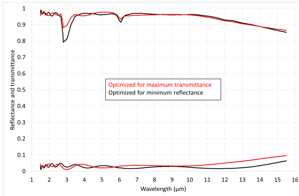
Fig. 11. Spectral performance of mid-IR antireflection coatings optimized for minimum reflectance (formula provided in Table 4) and maximum transmittance.
