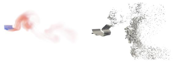
Fig. 5: Instantaneous overview of the simulations: volume rendering of the liquid volume fraction,  $\alpha_l$  high low (CEDRE (HR) - left) and level set in grey (ARCHER - right).
