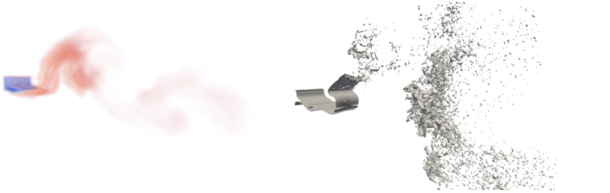
Fig. 5: Instantaneous overview of the simulations: volume rendering of the liquid volume fraction, \alpha_l high (CEDRE (HR) - left) and level set in grey (ARCHER - right).
