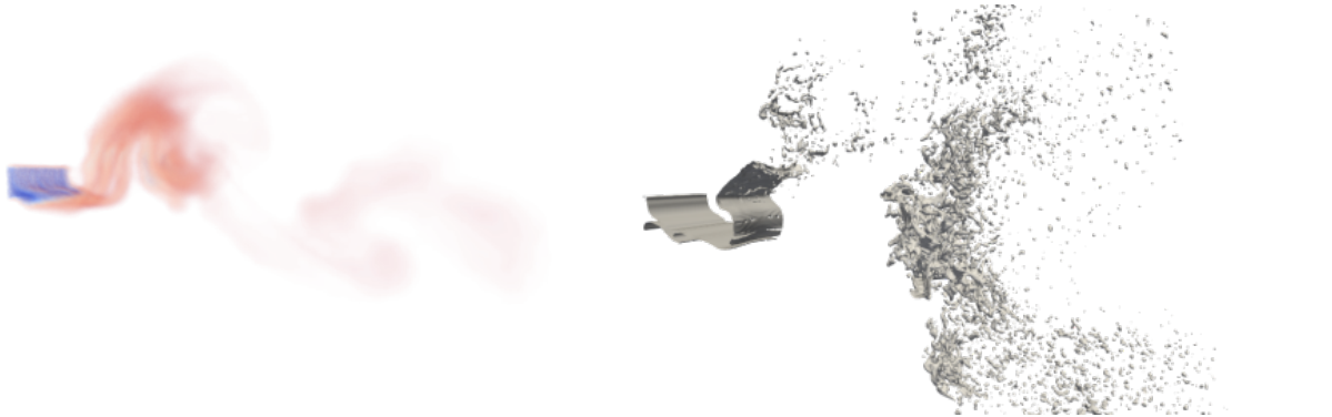
Fig. 5: Instantaneous overview of the simulations: volume rendering of the liquid volume fraction, \alpha_l high low (CEDRE (HR) - left) and level set in grey (ARCHER - right).
