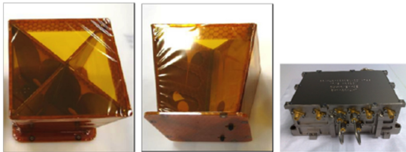
Fig. 11. SSR antenna and electronics box.
