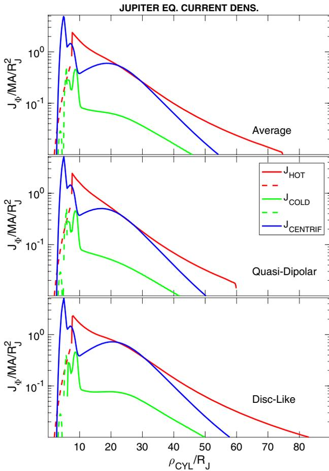
**Fig. 5.** Equatorial current density profiles of the Jovian magnetodisc models. Contributions associated with different forces on the plasma are colour-coded. Magnitude of current density is plotted (in units of mega-Ampères per squared planetary radius), with dashed curves indicating where current flows against the direction of planetary corotation.
