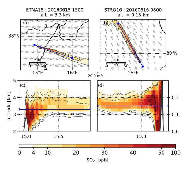
Figure 3. Simulated SO<sub>2</sub> concentration (ppb; colors) at 15 UTC on 15 June 2016 for ETNA15 flight (first column) and at 8 UTC on 16 June 2016 for STRO16 flight (second column) on horizontal (a,b) and vertical (c,d) cross sections (domain at 2 km resolution). Blue lines correspond to cross-sections locations. Grey arrows in (a) and (b) correspond to horizontal wind speed at the altitude of the cross sections.
