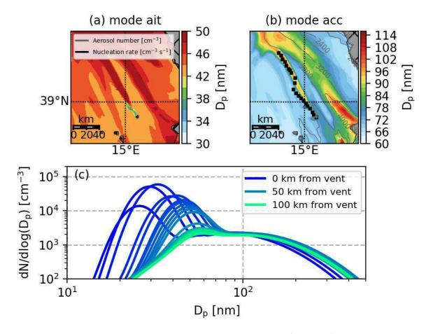
**Figure 7.** Spatial distribution of the simulated median diameter (nm; colors) at 8 UTC on 16 June 2016 at 150 m above sea level for mode iait (a) and mode jacc (b). Black squares correspond to points extracted to look at aerosol size distribution evolution (c). Evolution of the aerosol size distribution extracted along the volcanic plume (black squares on (b)).
