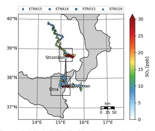
Figure 1. Track of the four SAFIRE-ATR42 flights : ETNA15 corresponds to 15 June 2016 flight around Etna (diamonds), ETNA16 to 16 June 2016 flight around Etna (dots), STRO15 to 15 June 2016 flight around Stromboli (squares) and STRO16 to 16 June 2016 flight around Stromboli (triangles). SO<sub>2</sub> concentration measured airborne are in colors [ppb]. Black lines correspond to the location of the two nested domains at 500 m horizontal resolution (Section 3)
