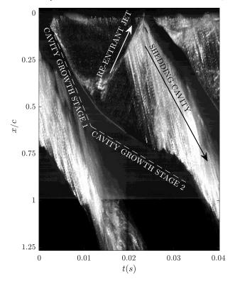
**Figure 5.** Space-time plot of a single shedding cycle of the rigid hydrofoil . showing the key components of the shedding cycle at  $\sigma = 0.8$ ,  $Re_c = 0.7 \times 10^6$  and  $\alpha = 6^\circ$ . The flow direction from top to bottom.
