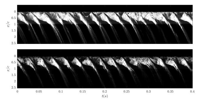
**Figure 6.** Chord-wise space-time plots from high speed images taken 100 mm along the span for the rigid (top) and flexible hydrofoil (bottom) at  $\sigma = 0.8$ ,  $Re_c = 0.7 \times 10^6$  and  $\alpha = 6^\circ$ . The flow direction is top to bottom.
