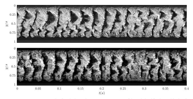
**Figure 7.** Span-wise space-time plots from high speed images 10 mm upstream of the mid-chord for the rigid (top) and flexible hydrofoil (bottom) at  $\sigma = 0.8$ ,  $Re_c = 0.7 \times 10^6$  and  $\alpha = 6^\circ$ . The flow direction is left to right.
