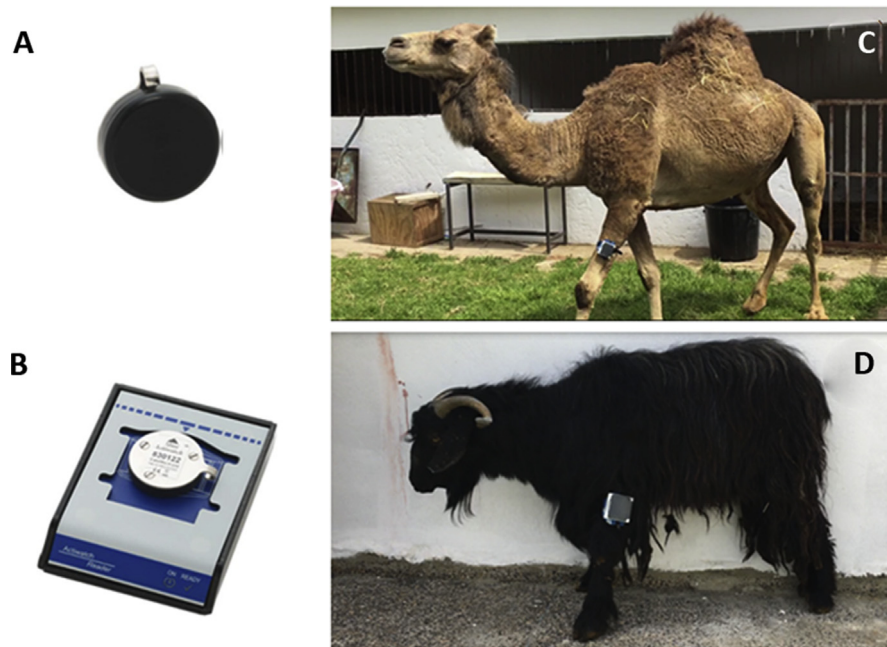
Fig. 1. Images of the piezo electric system used for the validation of the locomotor scoring method of LA rhythm. Actiwatch-Mini® device and its USB reader (A): the device and, (B): its USB reader, (C) and (D): Placement of the device on the lateral side of the forearm of the camel and of the goat, respectively.
