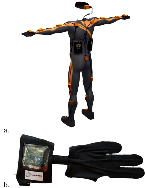
Fig. 1. Wearable sensors used in the experiment: (a) Xsens MVN suit; (b) e-glove from Emphasis Telematics.
