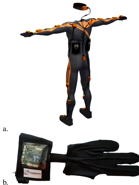
Fig. 1. Wearable sensors used in the experiment: (a) Xsens MVN suit; (b) e-glove from Emphasis Telematics.
