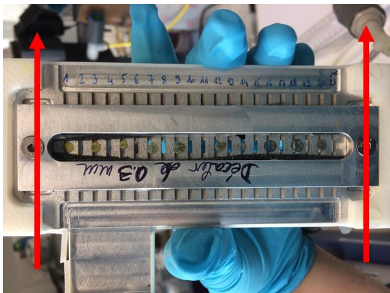
Figure S5. Photograph of the sample holder before SAXS measurement. The beam irradiated the sample perpendicularly to the substrate. The thin films composed of AuNR-Ag supercrystals were placed on a sample holder and scanned by moving the holder in respect to the SAXS beam in the direction of the arrow.
