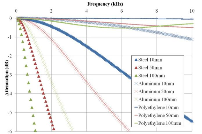
Figure 3: Acoustic attenuation of several materials as a function of frequency. The different curves are representing different materials ( $\blacktriangle$ : steel,  $\times$ : aluminum,  $—$ : polyethylene). For each marker the different colors represent different thickness (blue: 10 mm, red: 50 mm, green: 100 mm).
