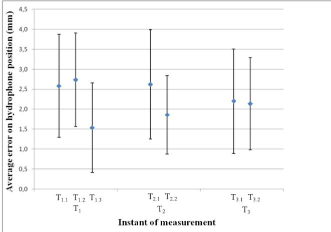
Figure 8: Average with standard deviation bars of three dimensional error between measured positions and reference positions of hydrophones, at different time of measurements. ( $T_1$ ): three measurements after array mounting. ( $T_2$ ): two measurements after test deployment in pool. ( $T_3$ ): two measurements after mission deployment in sea.
