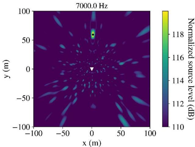
Figure 10: CBF map computed from simulated data at 7 kHz and a source at  $x = 2$  m,  $y = 59.5$  m.  $\blacktriangledown$ : array position at (0 m, 0 m, 53 m).  $\bullet$ : source position at (2m, 60 m, 24 m).
