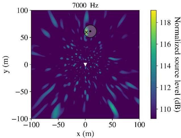
Figure 9: CBF map computed from the experimental data at 7 kHz.  $\blacktriangledown$ : array position at (0 m, 0 m, 53 m).  $\bullet$ : GPS boat position at (9 m, 61 m, 104m) (104m is the water depth).  $\times$ : estimated source position at (2 m, 60 m, 24 m). The uncertainty zone is represented by the whitened circle and has an 11.5 m radius.
