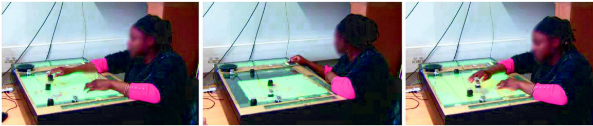
Fig. 3. Zooming with the keyboard interface: A participant selects a landmark in order to center it (left), then zooms in by pressing a key (middle), and finally explores the map once the robots are in place (right).
