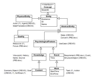
Figure 4: Unified Requirements Engineering meta-model.
