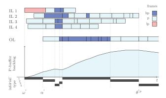
Figure 1: Example scenario. Ingress and egress frames at the top, buffer backlog as a function of time in the middle and interval types at the bottom
