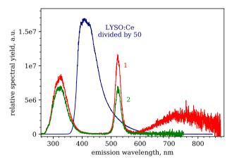
**Fig. 6** High-energy cathodoluminescence emission spectra of CdSe/CdS@PS 1% Curve (1) was recorded in the 0–200  $\mu$ s time gate and curve (2) between 0 and 32 ns time window relative to the excitation pulse. The CL spectrum of LYSO:Ce was recorded in 0–200  $\mu$ s time window
