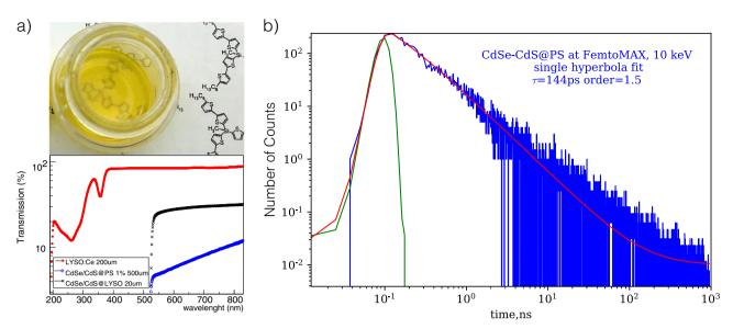
**Fig. 4** Scintillating kinetics of CdSe-based nanocomposite 1% weight concentration. **a** Transmission of CdSe/CdS nanocomposite 1% weight concentration 500 µm thick and CdSe/CdS drop-casted film with an effective thickness of 20 µm in comparison with LYSO:Ce crystal 200 µm thick. **b** Time-resolved decay kinetics of CdSe/CdS@PS 1% as measured at the FemtoMAX beamline with a IRF of 38 ps FWHM. The double-logarithmic scale has been chosen for better visualization of the data
