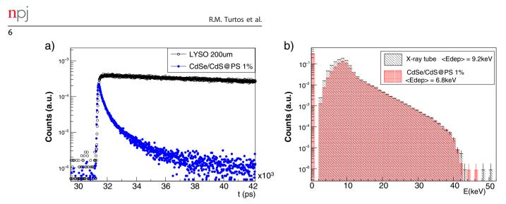
**Fig. 5** Two-step light yield determination of CdSe/CdS@PS 1% sample. **a** Comparative light output between LYSO and CdSe/CdS@PS 1% obtained in a time correlated single photon counting setup with a tungsten pulsed X-ray tube up to 40 kV. Data are shown within a 10 ns gate for visual purposes. **b** X-ray attenuation measured with the Timepix chip detector<sup>45</sup>
