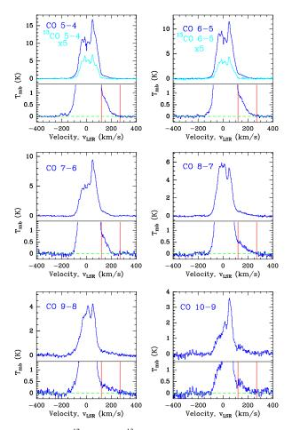
**Fig. 2.** Mid-J <sup>12</sup>CO and <sup>13</sup>CO lines observed with HIFI toward Sgr A\* (baseline subtracted). The two red vertical lines at  $v_{\rm LSR} \simeq +120$  and  $+270 \,\rm km^{-1}$  delineate the HPVW emission.
